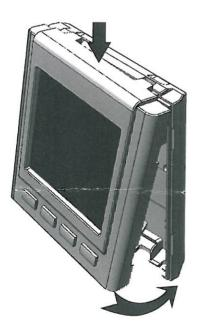
\* Attach the Thermostat Front to the Thermostat Back.
